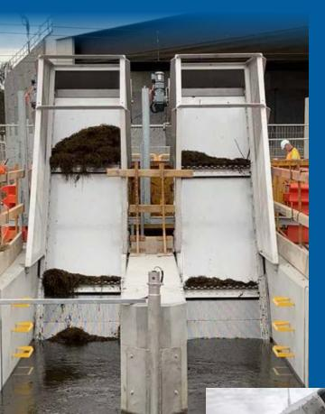
**AWMA** manufacture **Automated Trash Screens** that safely and effectively remove seeds, weed, rubbish and other debris from waterways.
