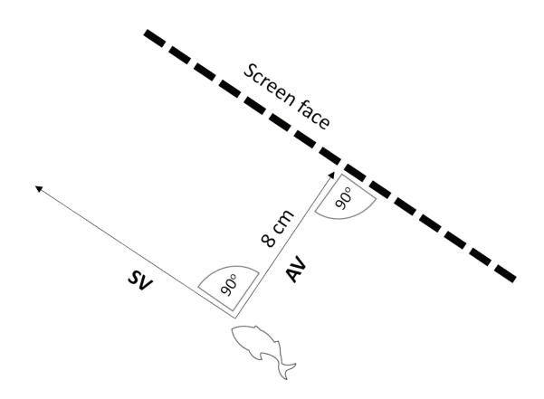
Figure 1. Approach velocity (AV) and sweeping velocity are to be measured 8 cm in front of the screen face.
